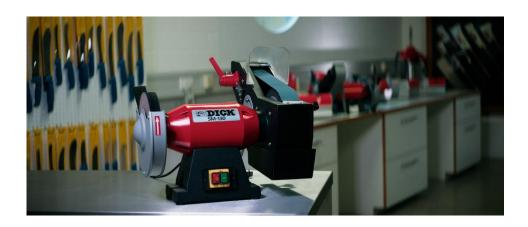
The F. DICK SM-130 wet belt grinding machine will be available from specialist retailers from July 2024 and is of course designed and built in accordance with the latest EU machinery directives. The powerful 300 watt motor with a direct drive is available in a 230 volt version.
